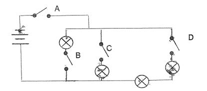
Which switches must be closed to light up two bulbs such that if one bulb fuses, the other remains lit?
