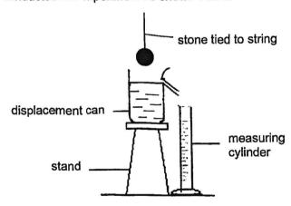
(a) What would happen when the stone was lowered into the above displacement can that was filled with water?
