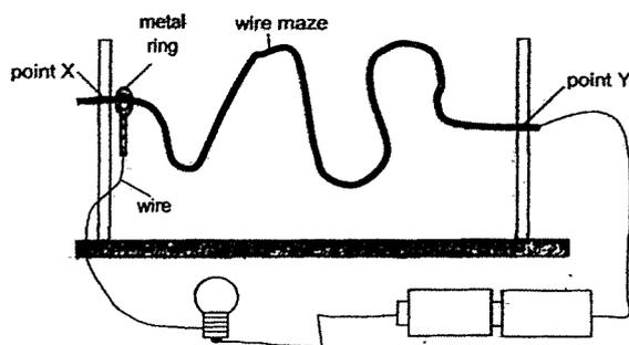
(b)(ii) The metal ring is a conductor of electricity. It will form a closed circuit which allows electricity to flow through hence lighting up the bulb.
