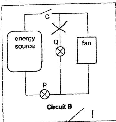
(a)(iii) If the bulbs fuses/fan is faulty, the electric current can flow through and form a closed circuit to allow the other to continue working.
