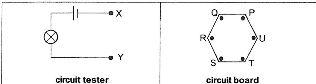
When the two points, X and Y, of the circuit tester are placed on two different points on the circuit board, the results are shown in the table below.
