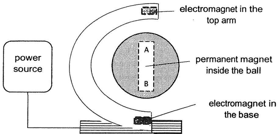
This toy makes use of the electromagnets in the top arm and the base, as well as a permanent magnet inside the ball.
