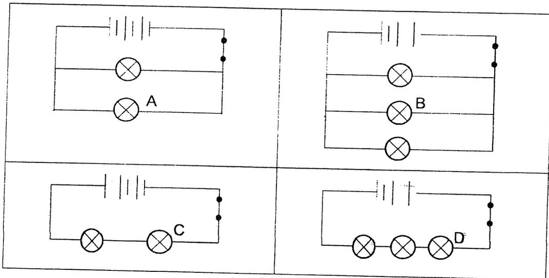
Which bulb(s) would be the brightest?
