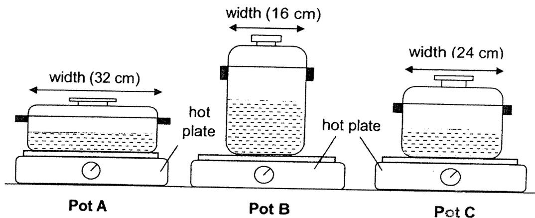
He started heating the pots of water on identical hot plates at the same time. He measured the time taken for the water in each pot to boil. His results are shown below.
